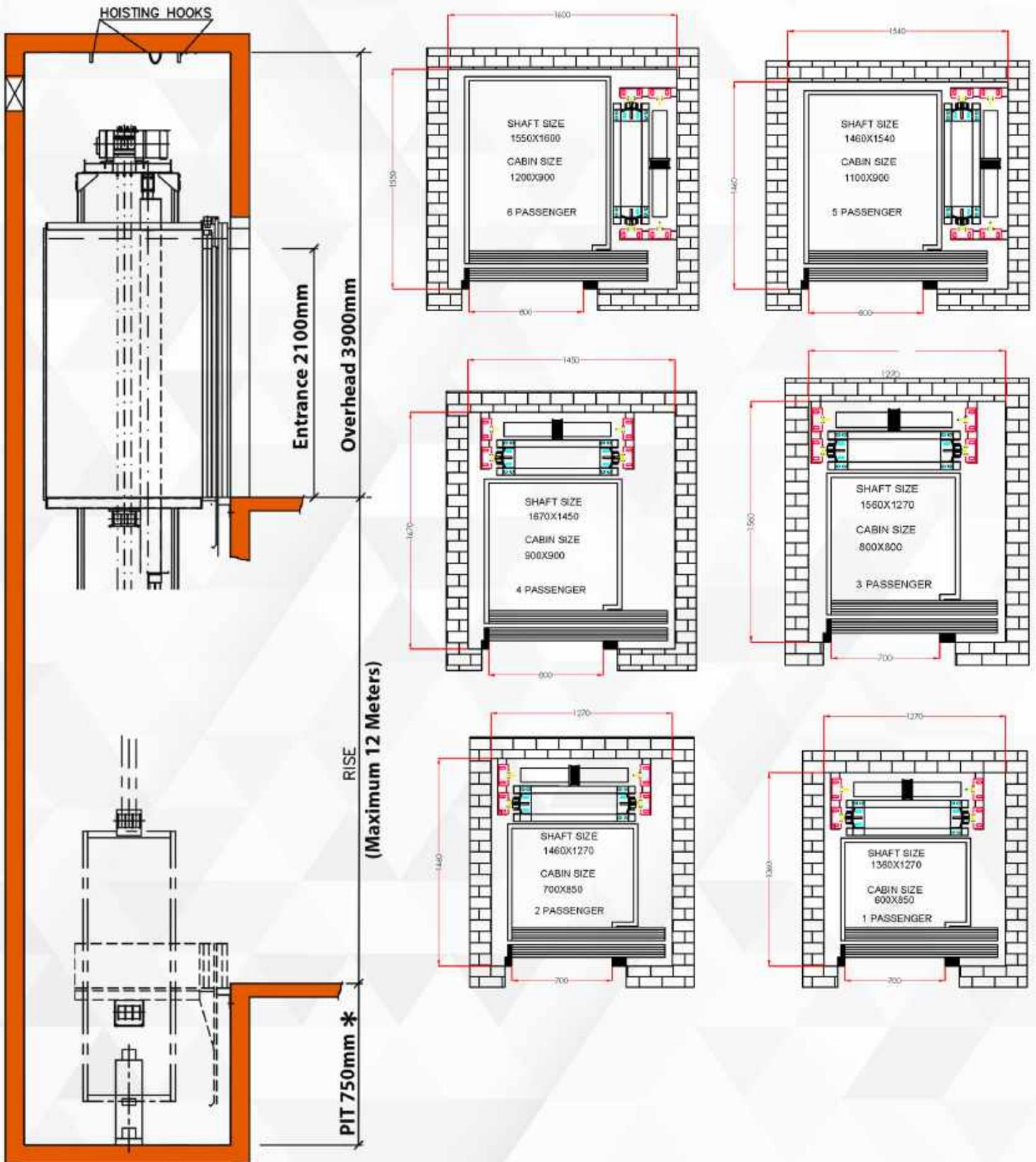
**Note:** Shaft dimensions changes with size of door and type of door opening ( Side Opening / Centre Opening )
